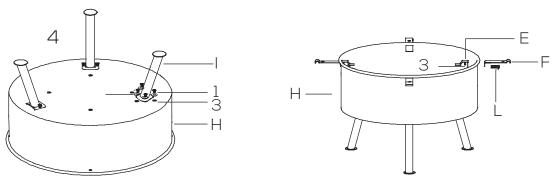
3. Join the two decorative rails(D) together and fit its joint into the arc slot of upper connectors(F), then put in the support plates(G), finally secure them with 1pc M 6 \*16MM bolts (2) and 1pc M6 nuts(3). Do the same for the other three parts.
