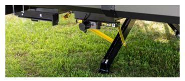
The PSx2 High-Speed Power Stabilizer adds several improvements to the PSX1. The dual motor design allows you to easily retract and extend the stabilizers with 50% faster operation over the competition and 30% more stable
