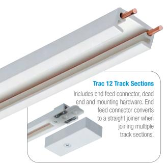
Trac 12 is the original miniature, surface mount, low voltage system that combines a 20-amp capacity with an extremely small, engineered-plastic profile. The system operates using remotely located or in-line 12-volt or 24-volt transformers. A maximum of 240 watts (12 volts) or 480 watts (24 volts) can be placed per circuit of track.
