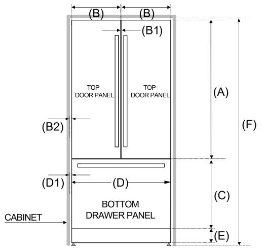
NOTE: The refrigerator comes with a 4" (100 mm) stainless steel toe kick installed to fit a standard 84" (2134 mm) tall cabinet niche.
