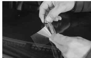
**NOTE:** When applying the curing film to the repair, no pressure is necessary. Just gently place it on glass and use a razor blade (3) to help the resin spread and remove the air bubbles inside.
