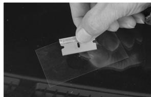
4. **Finishing:** Once the resin has fully cured, carefully remove the curing strip. Use the safety razor (3) to remove any excess repair resin. Use a clean cloth and solution to wipe away any fingerprints and smudges from the windshield. Your repair is complete.
