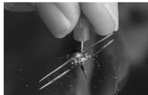
2. **Filling small pitted or scratched areas:** Remove cap from of Repair resin (1) and apply one or two drops into the damaged area. Quickly apply a Curing Strip (2) over the resin and damaged area. This will help hold the resin in place as it cures.
