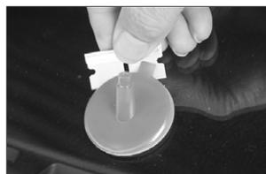
**11. Final pit filling:** Add a drop of repair resin onto areas where damage is still visible and quickly cover with a curing film (7). This will help hold the resin in place as it cures. When applying the curing film to the repair, no pressure is necessary. Just gently place it on glass and use a razor blade (8) to help the resin spread and remove the air bubbles inside.
