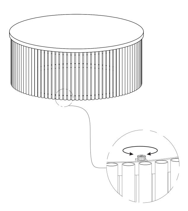
Note: Levelers on bottom of base can be adjusted if floor is uneven.
