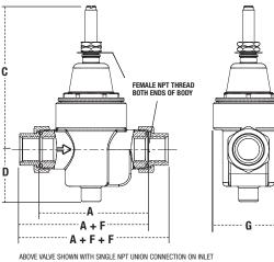
ABOVE VALVE SHOWN WITH SINGLE NPT UNION CONNECTION ON INLET VALVES MAY BE ORDERED WITH 0,1.02 UNION CONNECTIONS USING ANY COMBINATION OF NPT, SOLDER, PEX, QUICK CONNECT, CEF (F1960), PRESS OR CPVC CONNECTIONS REQUIRED "E" DIMENSIONS ARE APPROXIMATE ENGAGEMENT LENGTHS.
