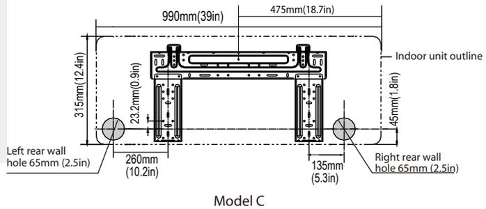
Correct orientation of Mounting Plate
