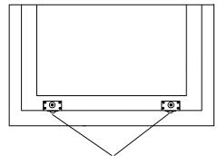
Note: Two rollers are located on the bottom of each door.
