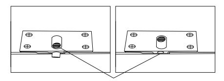
Step 2: If want to remove the doors, please push the pins upward, the pins will return back like above right picture, then you can remove the doors.
