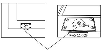
Step 1: Bottom rollers on sliding doors are equipped with adjustment to raise or lower the doors for proper operation and fit.
