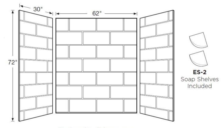
Designed to fit base areas 30" deep or smaller x 62" wide x 72 ½" high or smaller (762 mm x 1575 mm x 1829 mm)
