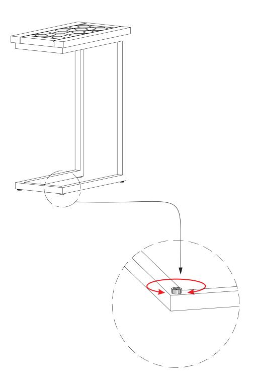
Note: Levelers on bottom of base can be adjusted if floor is uneven.
