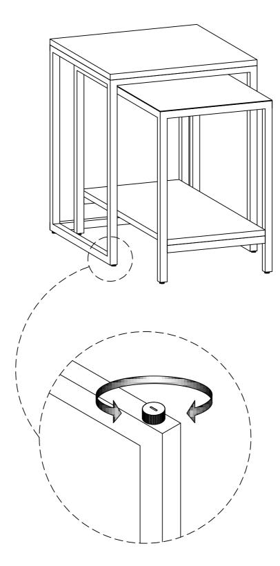
**Note:** Levelers on bottom of legs can be adjusted if floor is uneven.
