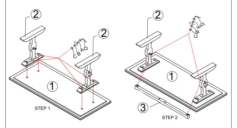
Step 1: Attach pedestals (2) to the top (1) by using bolts (A), lock washers (B) and flat washers (C). Do not fully tighten bolts at this step.
