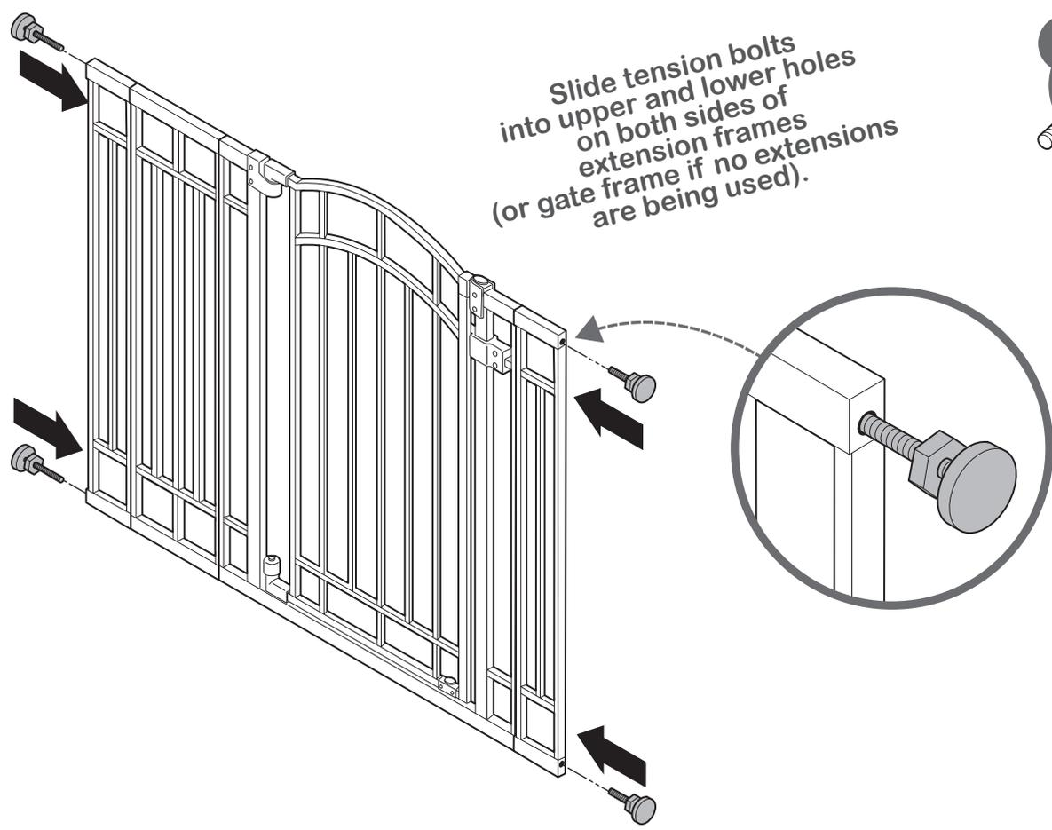
Slide tension bolts into upper and lower holes on both sides of extension frames (or gate frame if no extensions are being used).
