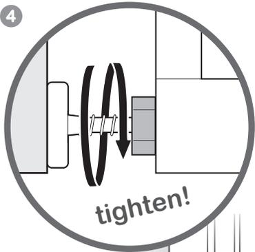
Use the tension nuts to tighten both of the bottom tension bolts.
