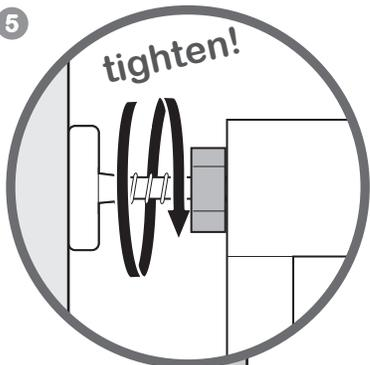
Use the tension nuts to tighten both of the top tension bolts.
