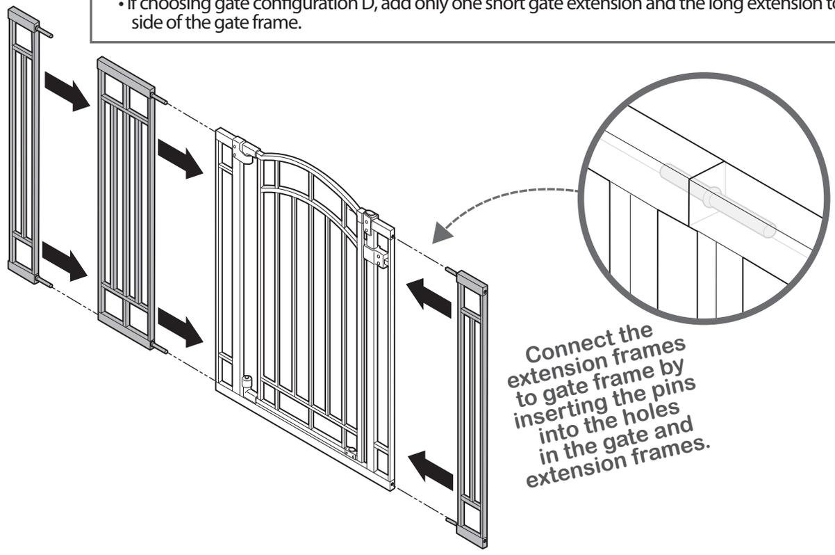
Connect the extension frames to gate frame by inserting the pins into the holes in the gate and extension frames.
