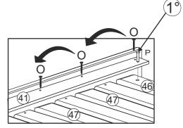
SECURE THE STRIP O WITH THE METAL PIN P. THAN PROCEED WITH FIXING THE SLATS
