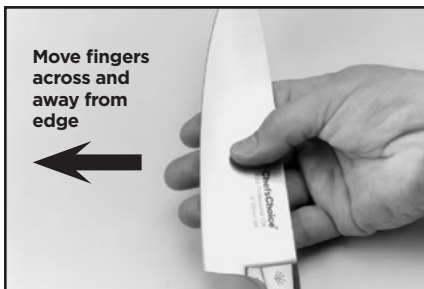
Figure 5. Burr can be detected by sliding fingers across and away from the edge. Caution! See text.
