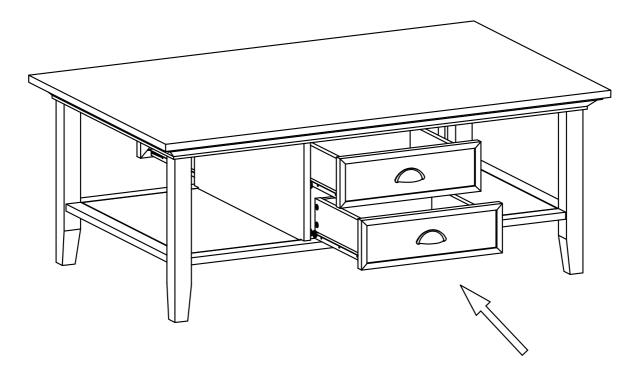
1. Insert assembled drawers into glides on assembled table.
