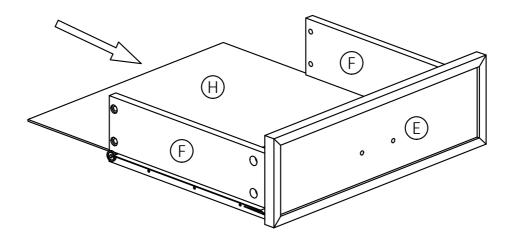
1. Slide Drawer Bottom (H) firmly into slots on Drawer Sides (F) and Drawer Front (E).
