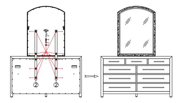
When using mirror only, hang the D Ring (G) onto the Hook (F).
