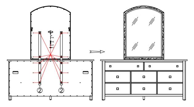
When using mirror only, hang the D Ring (G) onto the Hook (F).
