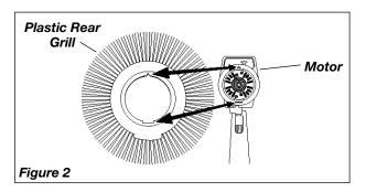
3. Fully seat *Plastic Rear Grill* and secure with *Plastic Nut* turning <u>CLOCKWISE</u>. (*Figure 3*)
