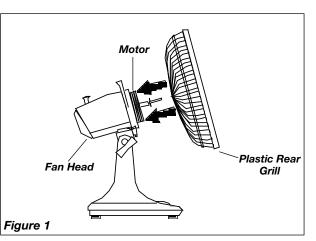
2. Align tab of *Plastic Rear Grill* with groove on top of front *Motor* cover. *(Figure 2)*
