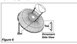
7. With Fan Head tilted back and centered, align *Ornament* of *Front Grill* so it is horizontal. Insert bottom of *Front Grill* into *Rear Grill*. *Tabs* at the bottom of *Rear Grill* should be between two wires of *Front Grill*. Snap *Front Grill* into the *Rear Grill* beginning at the top and working down both sides. *(Figure 7)*
