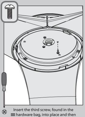
hardware bag, into place and the tighten all three screws.
