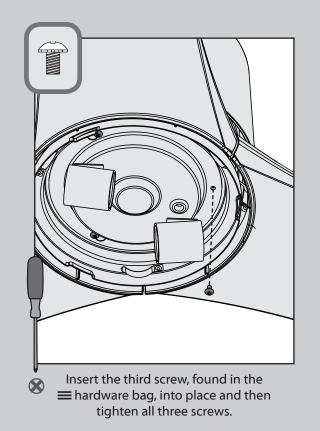
Make sure the light kit is securely attached to the mounting plate. Failure to properly secure all three assembly screws could result in the light fixture falling.
