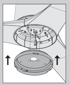
Thread theplug connector from the fan through the upper switch housing. Wrap keyhole slots around the screws and twist counterclockwise.
