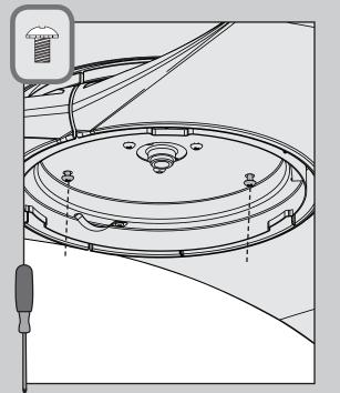
Screw two light kit screws from the hardware bag halfway into the switch housing housing. It does not matter which two screw holes you choose.
