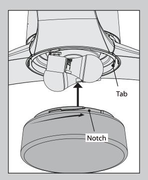
Lift the globe and align the notches in the globe with the tabs in the light kit. Attach the globe by lifting and twisting clockwise until it rests firmly in place.
