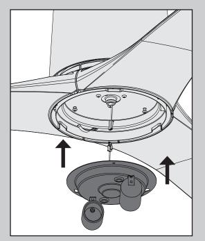
Connect the the plugs from the switch housing and the light kit. Push excess wiring into the switch housing. Wrap keyhole slots around the screws and twist counterclockwise.
