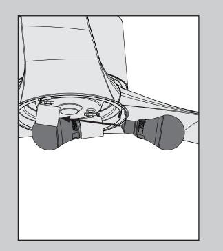
Install a light bulb in each socket. When necessary, replace with bulbs of the same wattage.
