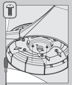
Screw two light kit screws from the ≡ hardware bag halfway into the motor housing. It does not matter which two screw holes you choose.
