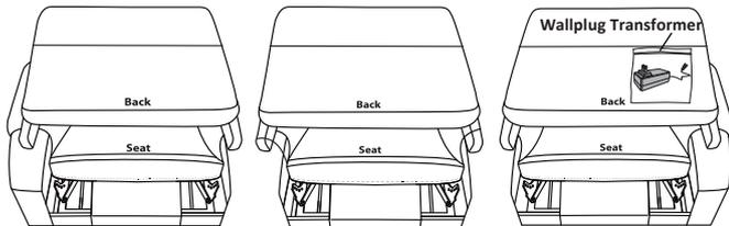
**Step2** Attach Backs: Position the LAF Back(A), RAF Back(B), Console Back(C) with the receivers positioned over the mechanism post on the Sofa body (D) as pictured below. Check to assure both sides of the mechanism post are positioned inside of the receivers on the back frame, push in a downward motion from the top of the back frame until a clicking sound is heard.
