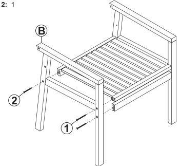
Align Right Arm (B) with the seat and stretcher. Use one M7x70mm Screw (2) to secure the back, and two M7x90mm Screws (1) to secure the front, as shown.
