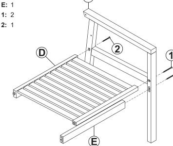
Align Seat (D) with Left Arm (A). Fasten the back of the seat using one M7x70mm Screw (2). Then, secure the front of the seat using one M7x90mm Screw (1).
