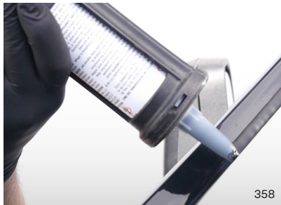
3M™ Polyurethane Glass Adhesive Sealant 590 is a fast curing one-component, high viscosity polyurethane sealant for bonding windshields and other substrates requiring high strength. This adhesive sealant is certified for 1 Hour Drive Away Time.
