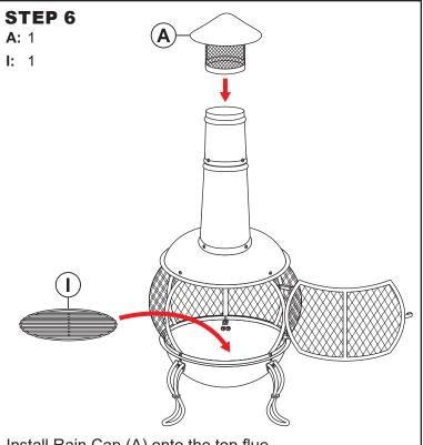
Install Rain Cap (A) onto the top flue. Place Log Grate (I) in the Bottom Bowl.
