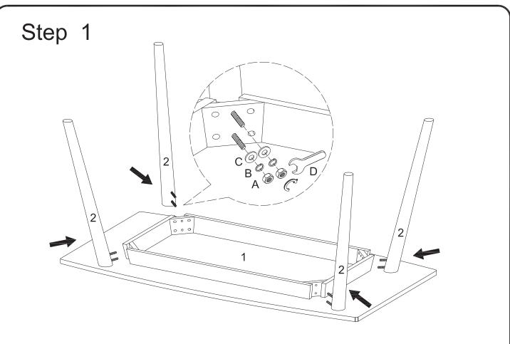
Attach the legs (2) to the table top (1) and secure it by using washers (C), spring washers (B), nuts (A) and wrench (D).
