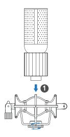
1. Mount the microphone onto the shockmount.
