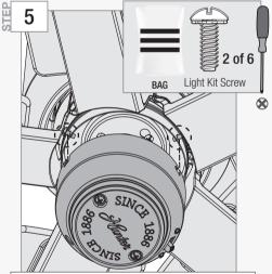
Partially install two of the light kit screws found in the  $\implies$  hardware bag. Align the notches in the sides of the lower switch housing with the screws on the upper switch housing. Twist the lower switch housing clockwise to lock into place.
