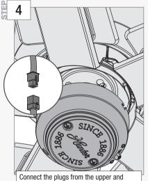
lower switch housings. Make sure to line up the colored markings on the connectors.
