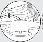
You must be able to secure the fan to building structure or fan-rated outlet box.
