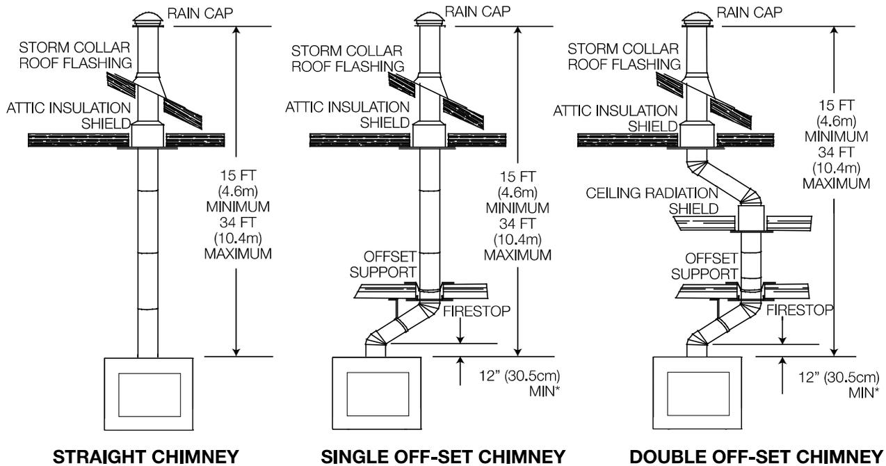
\* The first flue offset closest to the top of the appliance must be a minimum distance of 12" (30.5cm) from the top of the appliance.
