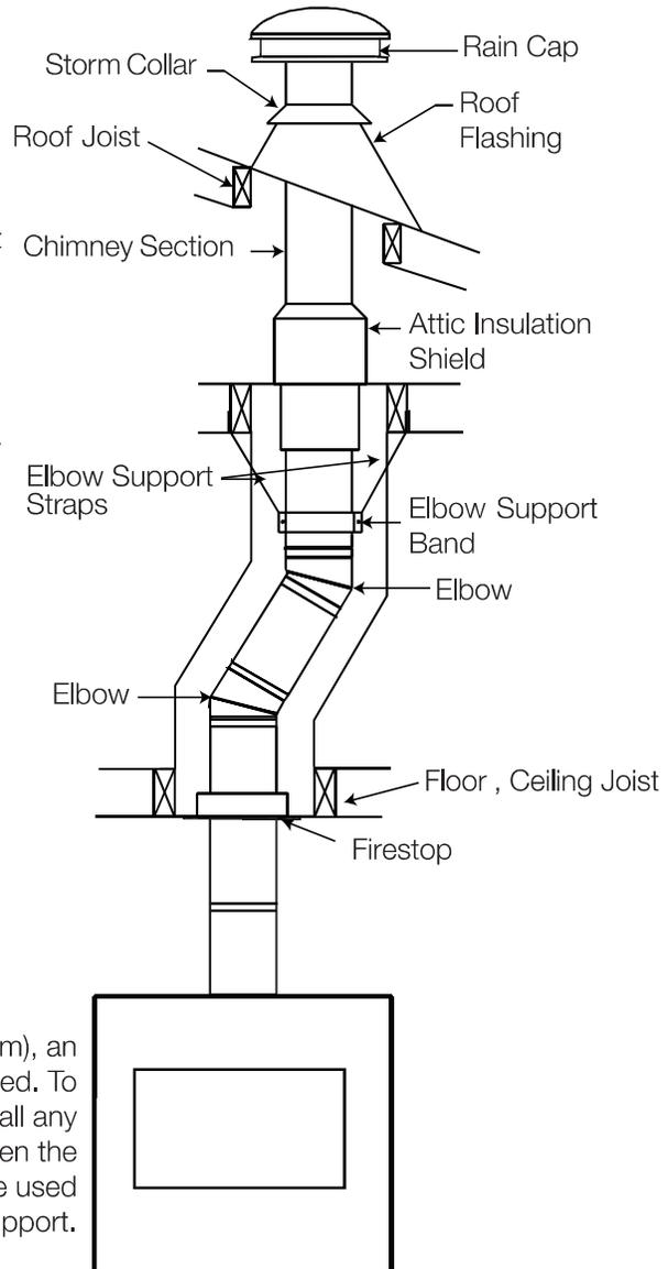
If the offset length is more than 36" (91.4cm), an intermediate support must be employed. To achieve longer offsets, you may install any available length of chimney pipe between the elbows. The intermediate support must be used in conjunction with an offset support.
