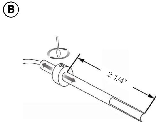
Set the depth to 2 1/4" and secure with set screw.
