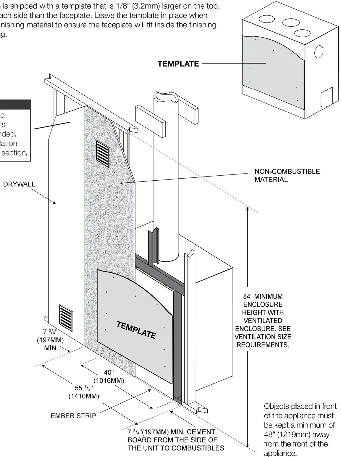
Objects placed in front of the appliance must be kept a minimum of 48" (1219mm) away from the front of the appliance.
