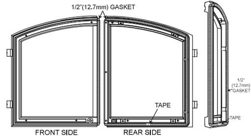
When you return to the other end of the gasket wrap a piece of tape around the other end of the gasket and cut through the center.
