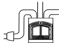
\* When installed with a masonry chimney, the hot air gravity and central heating system can only be installed off the sides.
