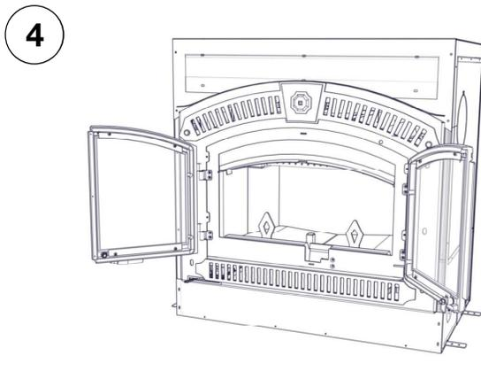
Press bypass rod downwards then inwards to lock into place.
