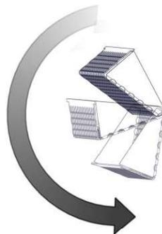
Reinstall perforated catalyst shield in reverse.
