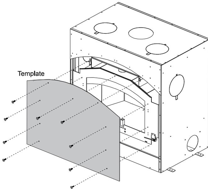
Remove the screws and template, discard only the template once all the facing material has been installed. Retain the screws for installing the faceplate.
