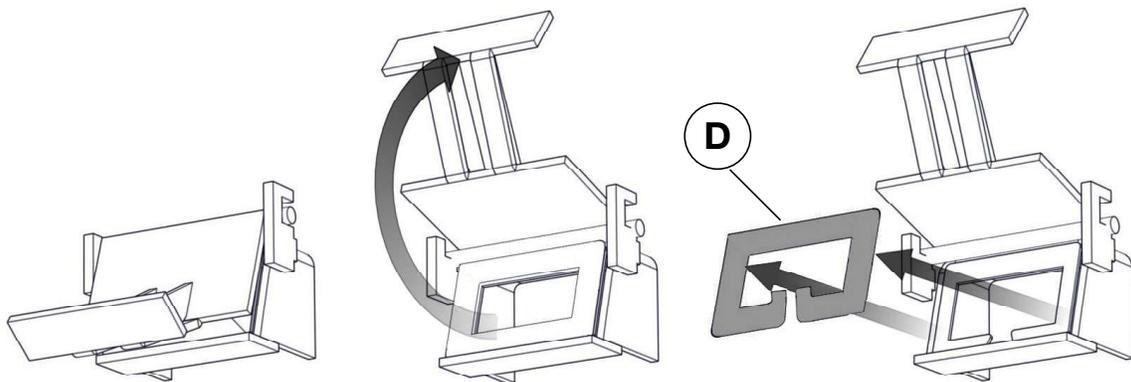
Open dilution door and remove gasket.
