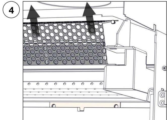
Move perforated catalyst shield up and over shoulder bolts.
