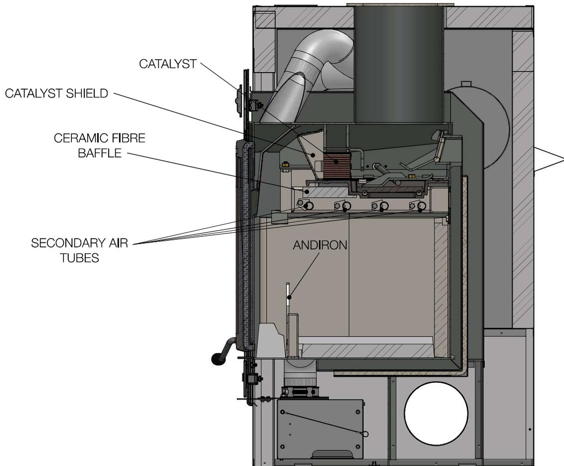
The TZ3000H contains a ceramic fibre baffle, catalyst and catalyst shield. It is important that each of these components are installed correctly prior to operating the appliance.
