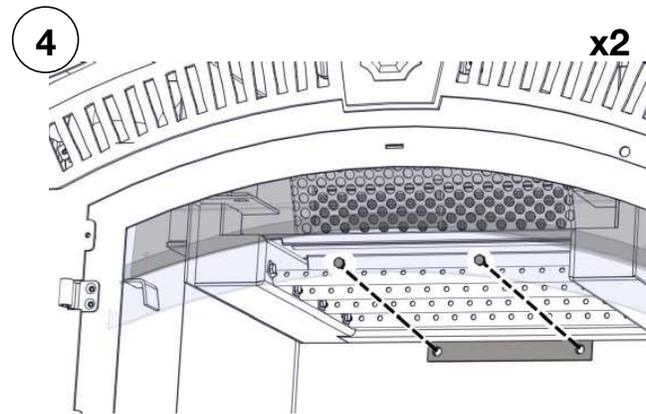
Remove front two nuts and bolts as illustrated above.
