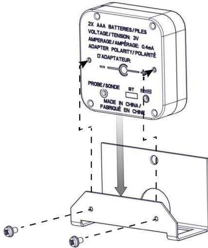
Slide the catalyst temperature monitor into the bracket and attach with screws (supplied).
