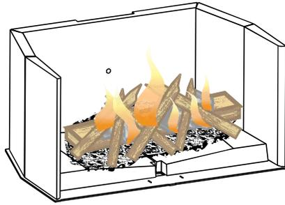
**E.** Slowly add larger wood (2x4 size pieces). Lay the pieces lengthwise from side to side in the hot coal bed with a shallow trench between, so that the primary air can flow directly into this trench and ignite the fuel above.
