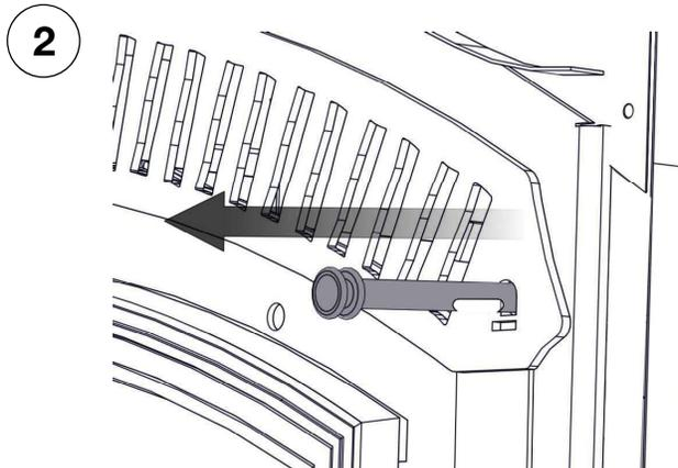
Ensure bypass door is open during startup and re-fueling. See above for bypass door rod location.
