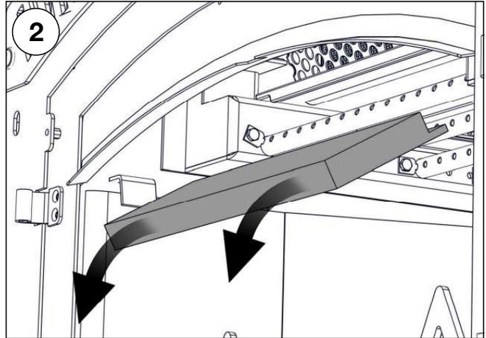
Slide baffle forward and down to remove.
