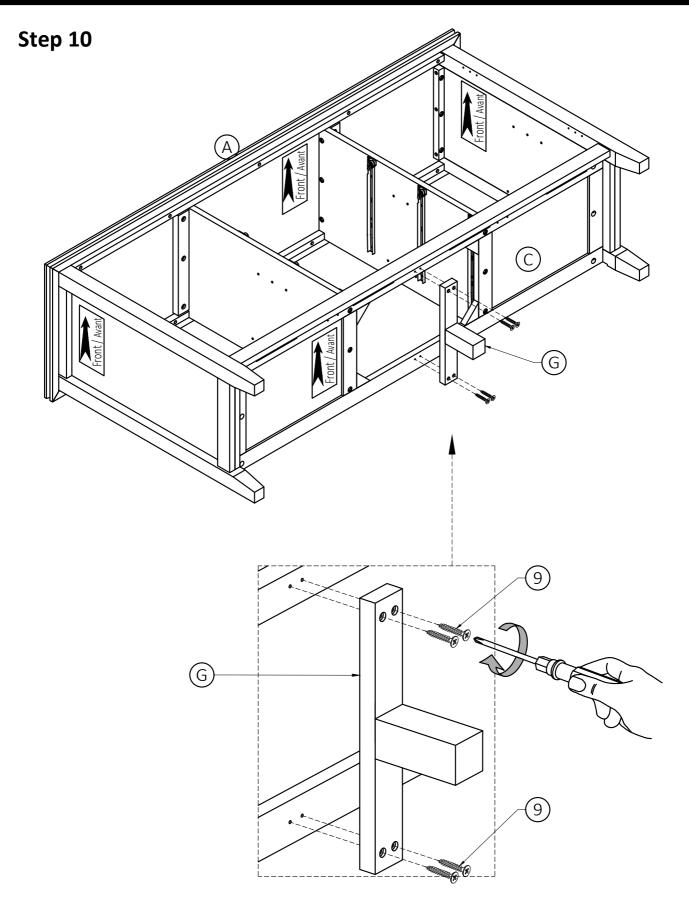
1. Align Bottom Support Leg (G) with pre-drilled holes on back of Bottom Shelf (C). Use Phillips Screwdriver to tighten four Phillips Screws (9).
