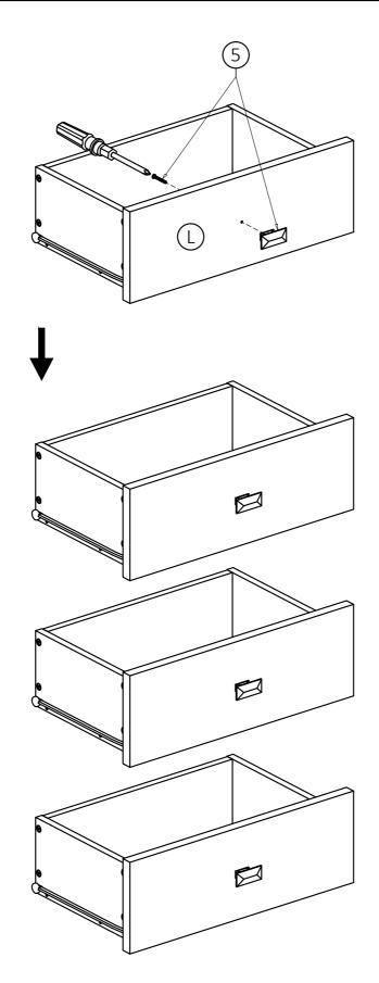
1. Use Phillips screwdriver to attach Handle (5) to Drawer Front (1).
