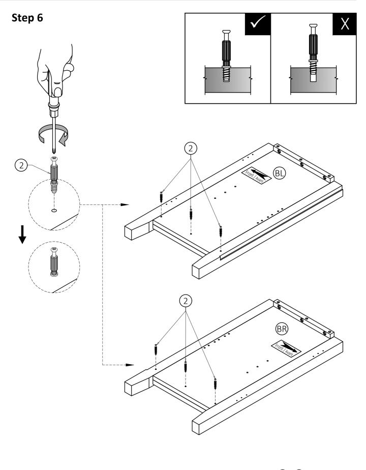
1. Attach three Cam Lock Pins (2) into pre-drilled holes on each part (BL), (BR). 2. Use Phillips screwdriver to secure Cam Lock Pins. Do not over-tighten.
