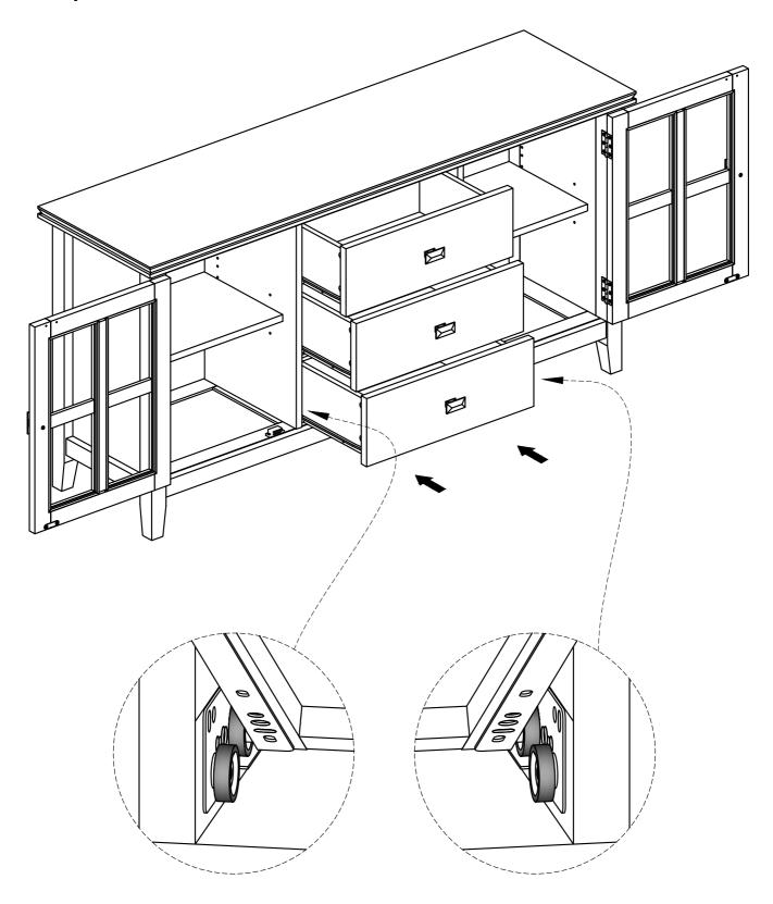
1. Insert assembled drawers into glides on assembled Sideboard Buffet.
