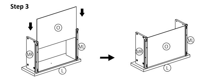
1. Slide Drawer Bottom () firmly into slots on Drawer Sides (ML), (MR) and Drawer Front ().
