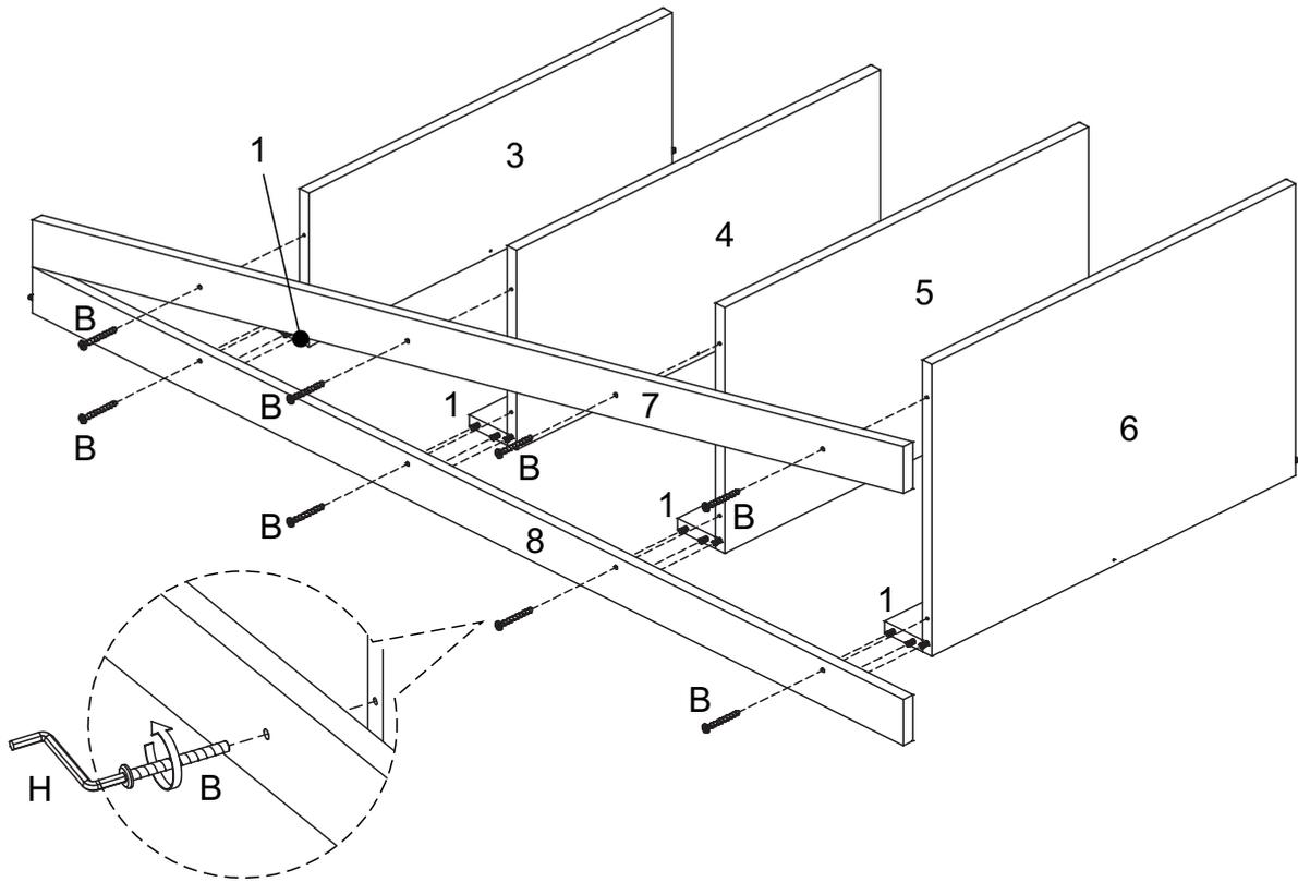
Attach the legs(7) and (8)to the shelves (3),(4),(5) and (6), secure it with the screws (B) and hex key(H).At same time,attach the back rails (1)to the legs (7) and (8), as shown.
