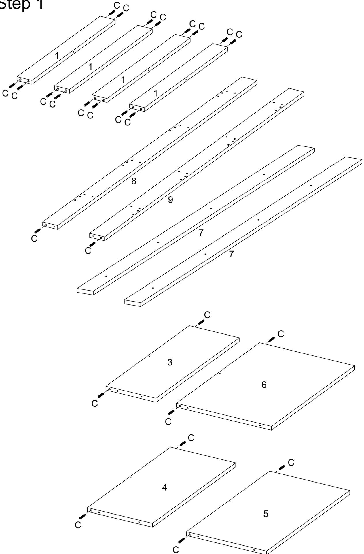
Insert wood dowels (C) into the indicated parts.
