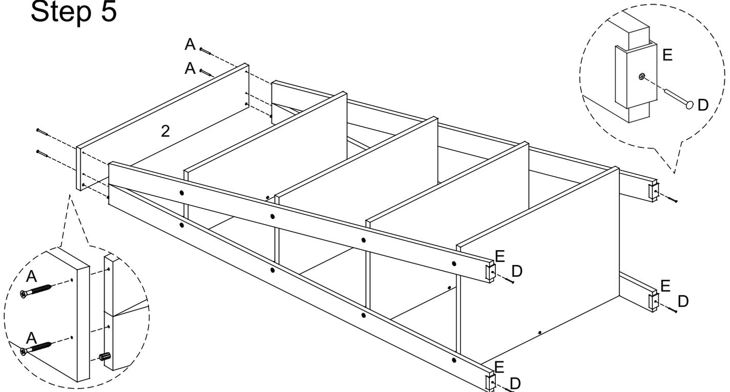
First, attach the top panel(2) to the unit, secure it with screws (A). After, attach the plastic feet (E) to the pre-assembled legs and secure it with nails (D).
