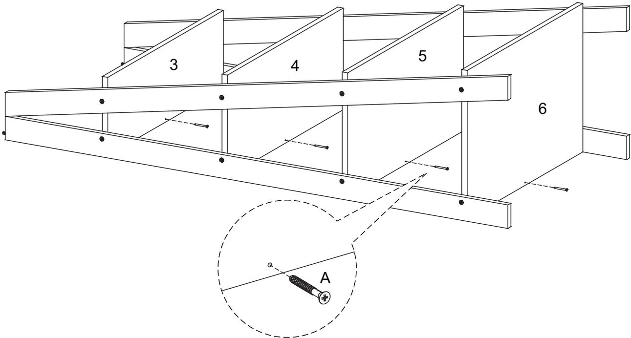
Attach the back rails (1) to the shelves (3), (4), (5) and (6), secure it with the screws (A) and a phillips headscrewdriver (not included), as shown.
