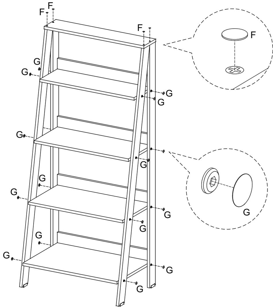
Use plastic cap (F) to cover screw heads (A) as desired. Use plastic cap (G) to cover screw heads (B) as desired.
