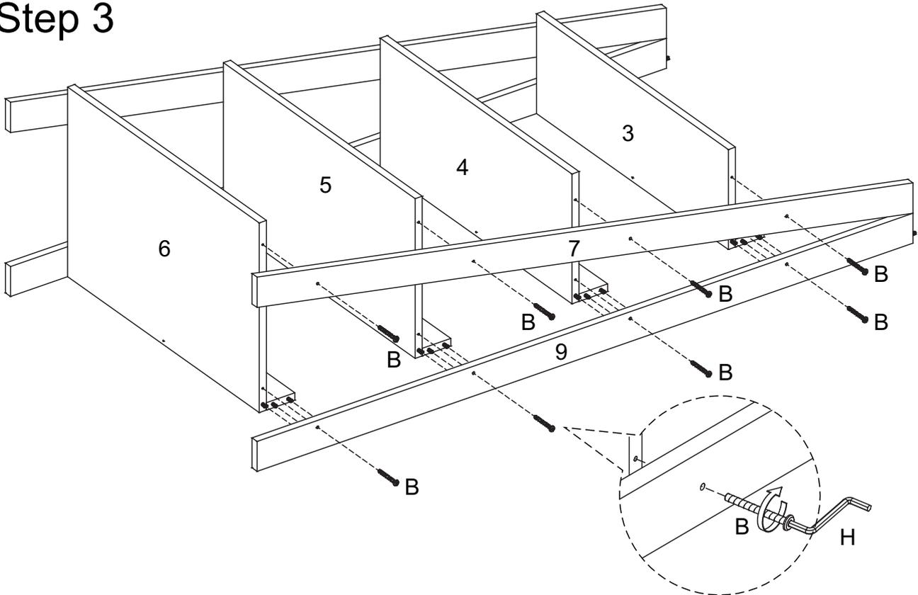
Attach the legs(7) and (9)to the shelves (3),(4),(5) and (6), secure it with the screws(B) and hex key(H).At same time,attach the back rails(1) to the legs (7) and (9), as shown.
