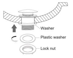
2. Install washer, plastic washer and lock nut from below. Secure the pop-up by tightening the lock nut.
