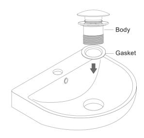
1. Install the pop-up body and gasket into the drain hole.
