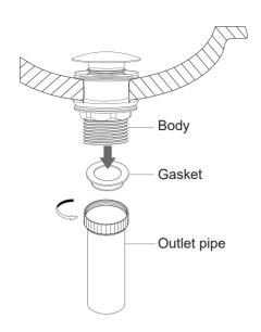
3. Install the pipe with the gasket inside.
