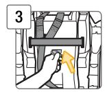
Rotate Metal Retainer and Push It Up Through Shell and Pad
