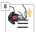
From Top of Seat, Pull Buckle Out of Shell and Pad
