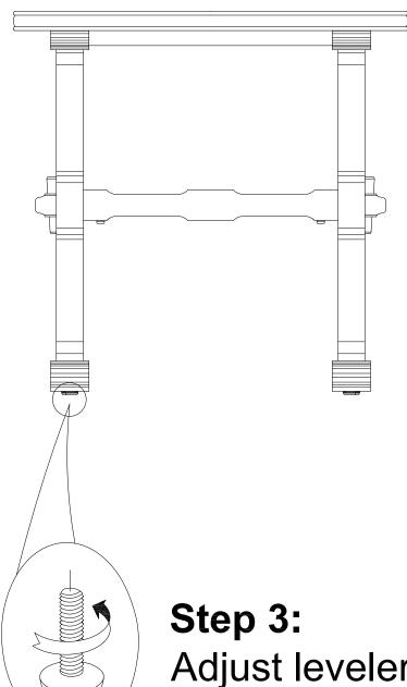
Adjust leveler if needed to level table on uneven floor.
