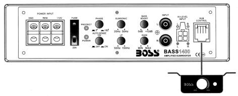
Subwoofer Remote Control allows you raise or lower the level of the subwoofer.
