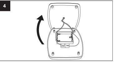
Carefully lift the bottom of the panel, ensuring the wires remain intact. Gently remove the old batteries. Paying attention to the positive and negative terminals, insert new batteries.
