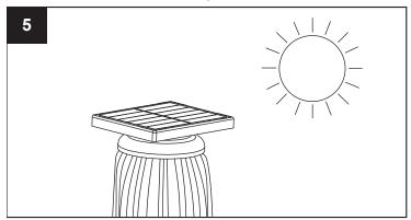
Before the first use, ensure the solar panel receives at least 8 hours of direct sunlight to charge the batteries.
