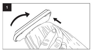
Twist the solar panel counterclockwise and gently lift the panel off the umbrella. Take care not to pull on the wires.
