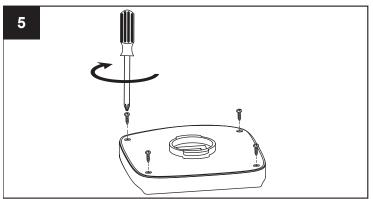
Carefully replace the bottom of the panel and align the screw holes. Secure the panel with the screws removed in step 3. Do not over-tighten the screws.
