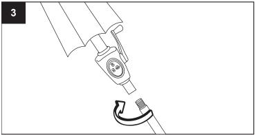
Align the threaded end of Pole (B) with Umbrella (A) and twist the pole to firmly secure. Some force may be required to ensure the poles thread together.
