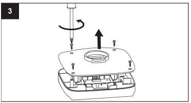
Place the solar panel face-down on a soft, clean surface. Remove (4) screws from the bottom of the panel.
