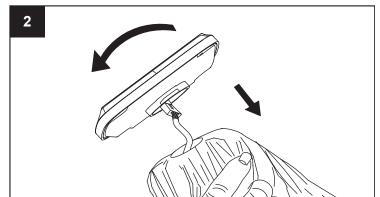
Align the tabs on the solar panel with the notches on the top of the umbrella, ensuring the connectors and wires are fully inside the hollow space. Turn the solar panel clockwise to lock in place; do not over-tighten.
