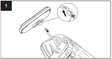
Firmly, but carefully, align and attach the connector on the solar panel to the connector on the top of the umbrella. Do not pull on wires, as doing so may permanently damage the wiring connections.
