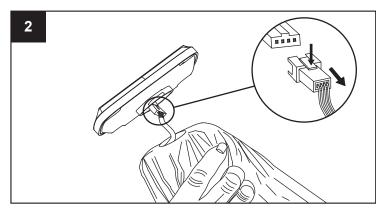
Carefully disconnect the plug from the socket by pressing the tab on the connectors. Gently pull apart by holding the plugs, never pull on the wires.
