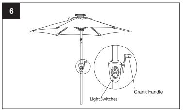
Turn the crank handle clockwise to open the umbrella canopy. Press the light switch above the crank handle to turn the solar lights on/off. Keep lights off during the day to preserve battery power.
