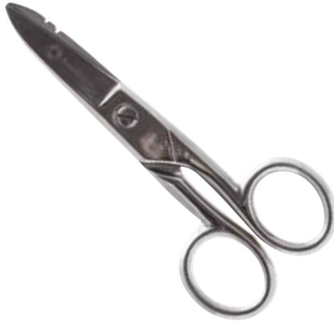
Unlike regular scissors or shears, the serrated blades keep wire from slipping out of the jaws, so that cutting through hardware cloth, cable, wire netting, and other difficult-to-cut materials becomes an easy task.
