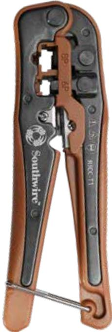
This all-in-one tool cuts and strips both phone and data cable. It also crimps RJ45 (data) as well as RJ11/RJ12, and RJ22 (phone) modular plugs.
