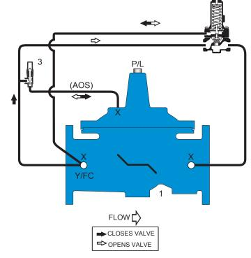
toward a closed position, sustaining pressure in the upstream zone. The valve will close, if necessary, until upstream pressure is above the pilot setting. The valve should be specified to include the optional opening speed control and position indicator when used for Pressure Sustaining applications.
