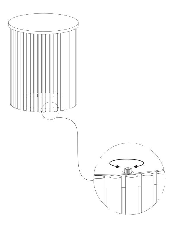
Note: Levelers on bottom of base can be adjusted if floor is uneven.
