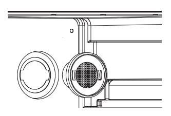
Rotate filter 1/4 turn to lock in place
