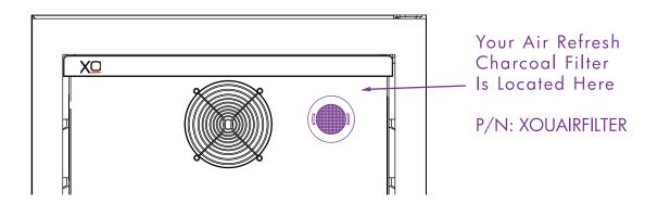
Rotate the filter 1/4 turn to unlock
