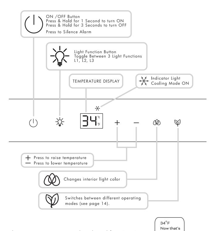
The temperature setting can be adjusted from 34-50°F. Your controls are simple and intuitive to operate.
