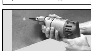
Drill 1/2" pilot hole using Greenlee Kwik-Stepper<sup>®</sup> step bit.
