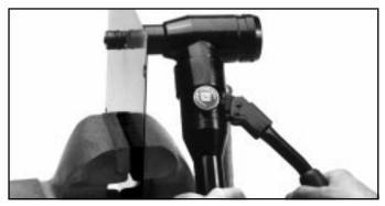
Turn the release valve knob clockwise. Rotate driver to best operating position, and then pump lever handle until the punch is completely through the material.
