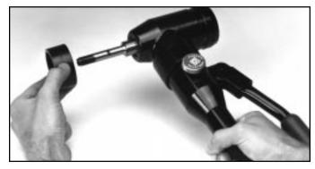
3. Thread 7/16" draw stud tightly into driver. Place the die on the draw stud.
