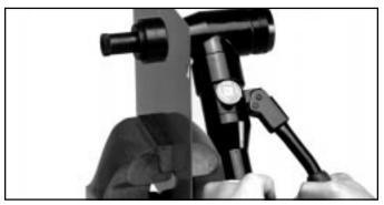
Turn release valve knob clockwise. Pump lever handle until the punch is completely through the material.
