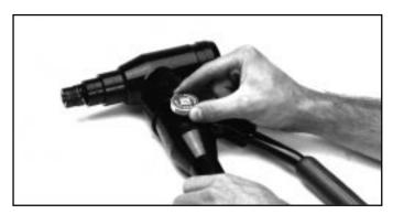
5. Release by turning release valve knob counterclockwise and remove the punch, die, adapter and draw stud.
