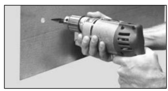
Drill 1/2" pilot hole using a Greenlee Kwik-Stepper® step bit.
