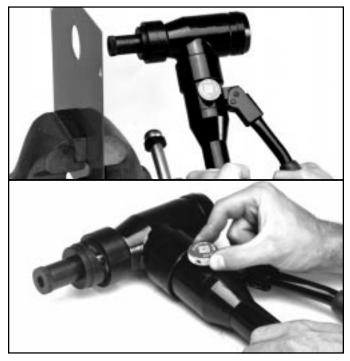
Release by turning the release valve knob counterclockwise.
