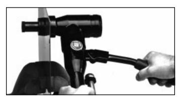
6. Make sure draw stud threads are fully engaged in the adapter.
