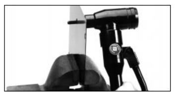
2. Turn the release valve counterclockwise to make sure the ram is fully extended. Install 3/8" draw stud, 3/4" x 3/8" adapter, spacer and 1/2" conduit die and insert into pilot hole.
