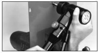
4. Turn the release valve knob counterclockwise, to make sure the draw stud is fully extended. Insert stud through pilot hole.
