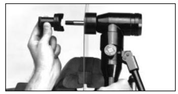
5. Thread the adapter with punch onto the draw stud.
