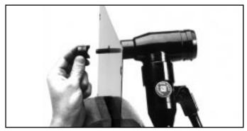
Thread 1/2" conduit punch onto draw stud until the punch is tight. Make sure the draw stud threads are fully engaged in the punch.
