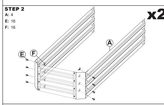
**IMPORTANT:** One end of the side panels has double mounting holes, install the single-hole side to the corners.
