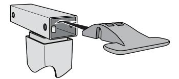
2. Insert release lever with rounded side up into the column assembly over pin.
