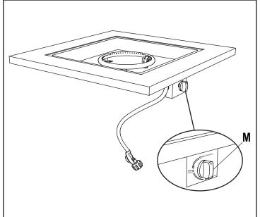
1. Check and confirm that Control Knob (M) for the gas supply system is turned to the "OFF" position before starting assembly.
