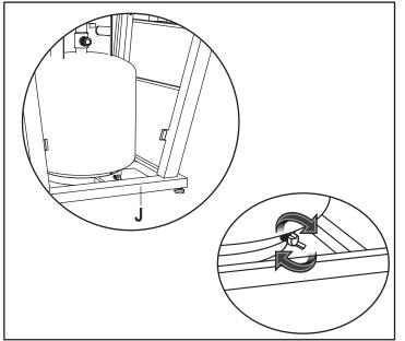
1. Place propane tank (not included) into Metal Stand (J). Make sure the gas tank sits on Metal Stand (J) entirely and securely. Turn the preassembled wingnut screw on the outer part of Metal Stand (J) clockwise to secure the propane tank tightly.
