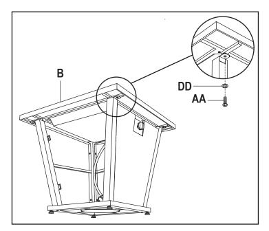
4. Gently place Table Top (B) onto the assembled base. Fasten Table Top (B) to the base using four M6 x 12 Bolts (AA) and four Washers (DD).
