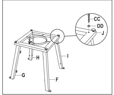
Attach Left Back Leg (F), Left Front Leg (G), Right Back Leg (I) and Right Front Leg (H) to Metal Stand (J) using four M6 x 40mm Bolts (CC) and four Washers (DD).
