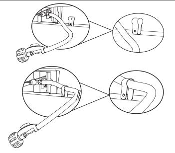
5. Attach the regulator hose tightly to the bracket on the inside of Front Panel (D).
