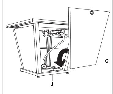
6. Insert the pins on the bottom of Door (C) into the holes on the open side of the assembled base.
