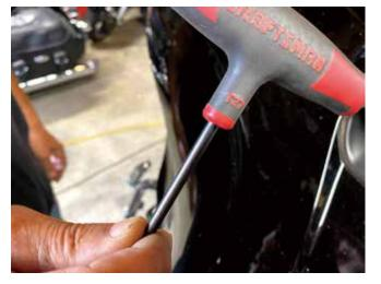
3. Remove (2) T-27 Torx bolts from outer edges of inner fairing near the fork tubes (facing forward) 4. Remove (3) T-27 Torx bolts from bottom edge of windshield.
