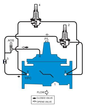
Reducing Valve, causing it to throttle toward closed, allowing the Low Flow By-Pass to resume command of flow and pressure.
