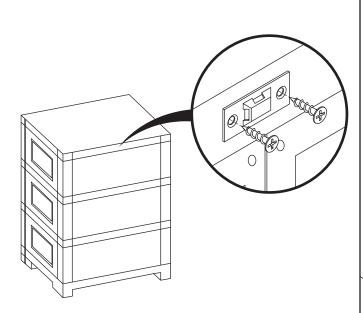
Secure one mounting tab to the back of the top panel using the short screws.
