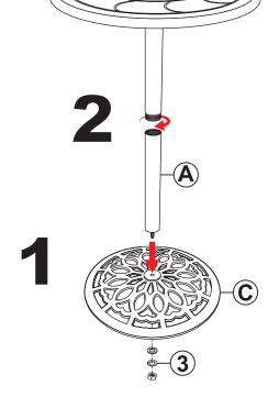
Firmly secure Lower Pedestal (A) to Base (C) using 12mm Washers/Nut Set (3).
