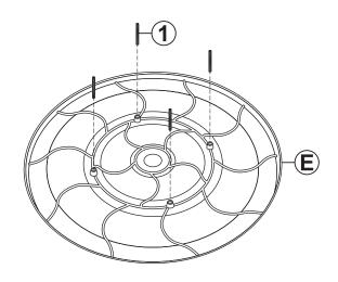
Firmly install four Grub Screws (1) into the underside of Tabletop (E) using the included Hex Key.
