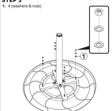
Secure the pedestal to the tabletop using the rest of Grub Screw Sets (1), as shown.
