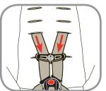
**a.** From the front of child restraint, pull harness straps out of the upper harness slots.
