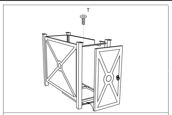
4. Hang the bottom (H) of the door plate on the round bracket. Top with 1PC screw(T)lock.
