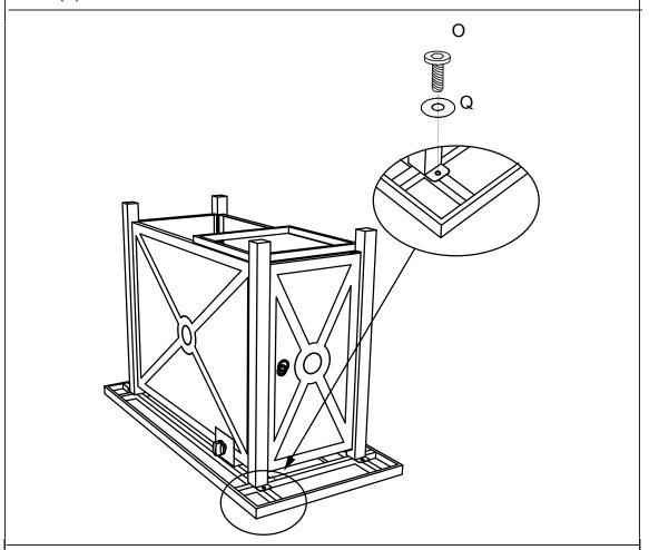
5.Attach the assembled base to the bottom of top using 4pcs of screws (O), and 4pcs M6 washers(Q), make sure the panel (L) faces the valve stem. Tighten all screws.
