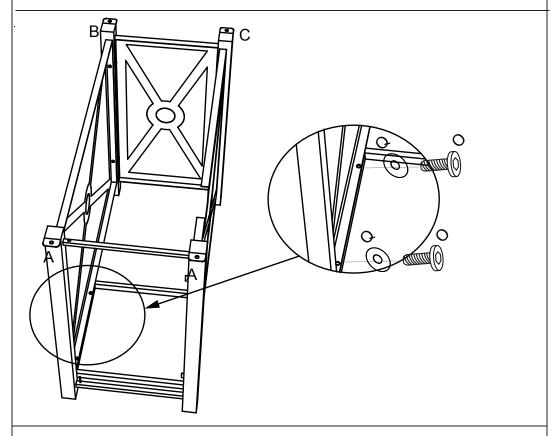
2. Connect the tank holder/base (I) With table Lets(A/B/C) by 4pcs screws (O) and 4pcs M6 washers(Q).
